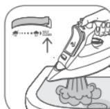
Fill the water tank with untreated tap water up to the max mark and heat the iron to the temperature. Unplug the iron and hold it over a sink horizontally. Hold the steam control into the Self Clean position : steam will now begin to build up. After a few seconds water will emerge from the soleplate, rinsing dirt and scale particles out of the steam chamber.
