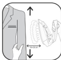
Hold down the burst of steam button and place the iron a few inches away from the garment to avoid burning delicate fabrics.
