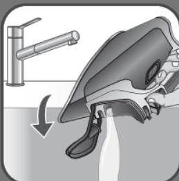
Empty the water tank over a sink (the iron is unplugged).
