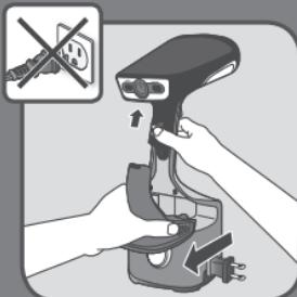
**EN** Unlock and remove the water tank.
