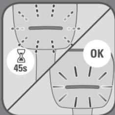
**EN** Wait until the light stops flashing (approximately 45 seconds).
