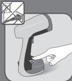
**EN** Press the water tank locker.
