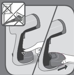
**EN** Press the water tank locker.
